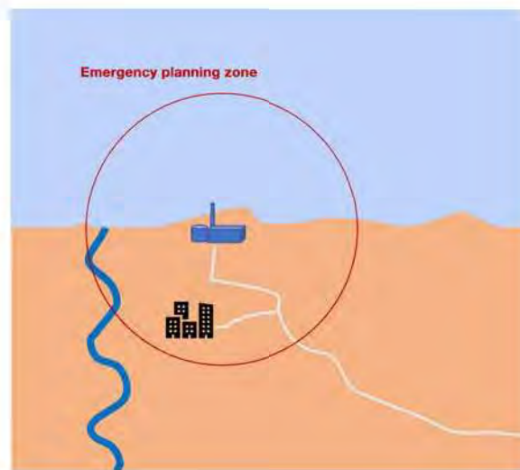
FIG. 2. Example of a site with a physical barrier (river) preventing construction of an alternative evacuation route in another direction. The site is unsuitable unless a bridge is constructed or an alternative evacuation route is made available.
