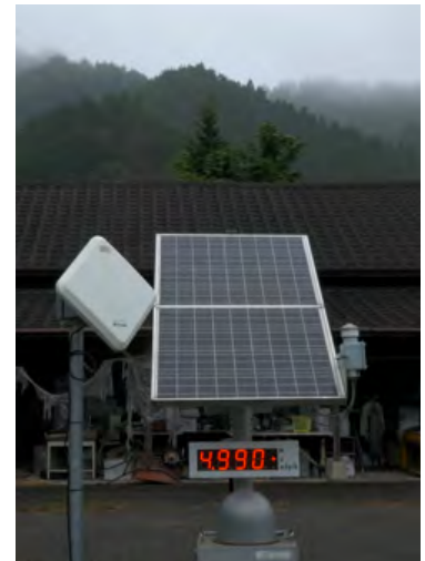
Radiation monitoring station
