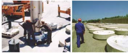
Intermediate level nuclear waste is inserted into in-ground storage containers at the WWMF
