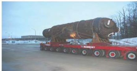
A steam generator is transported to the WWMF for interim management
