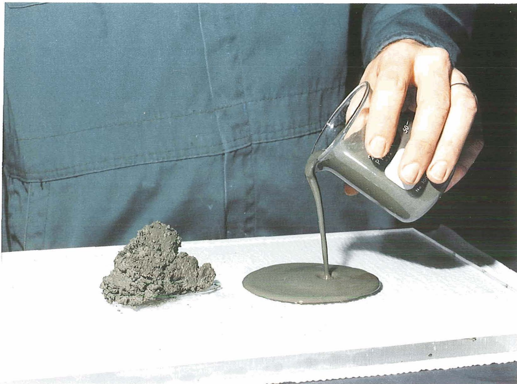
FIGURE 4-9: Mixture of 90% Type 50 Portland Cement, 10% Silica Fume at a Water-to-Solids Ratio of 0.4 Without Superplasticizer (left), and with 0.75% Superplasticizer (right)
